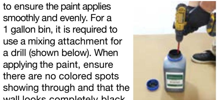
When applying the shielding paint, verify regularly that you are applying at your predetermined rate of wall space. The paint will not reach its maximum shielding capacity until completely dried, which depending on the environment can take between 24 to 48 hours.
